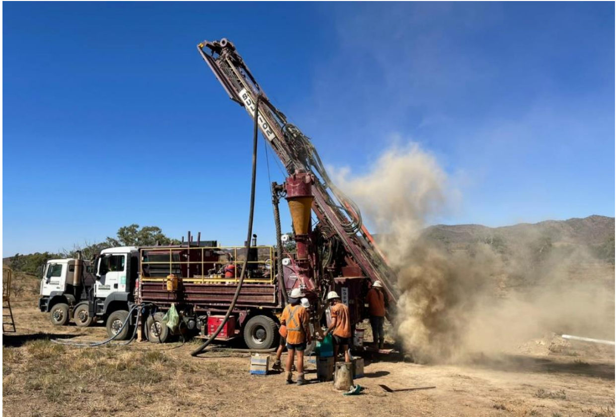
Figure 3: RC Drillhole being collared at the Wyacca Prospect.
