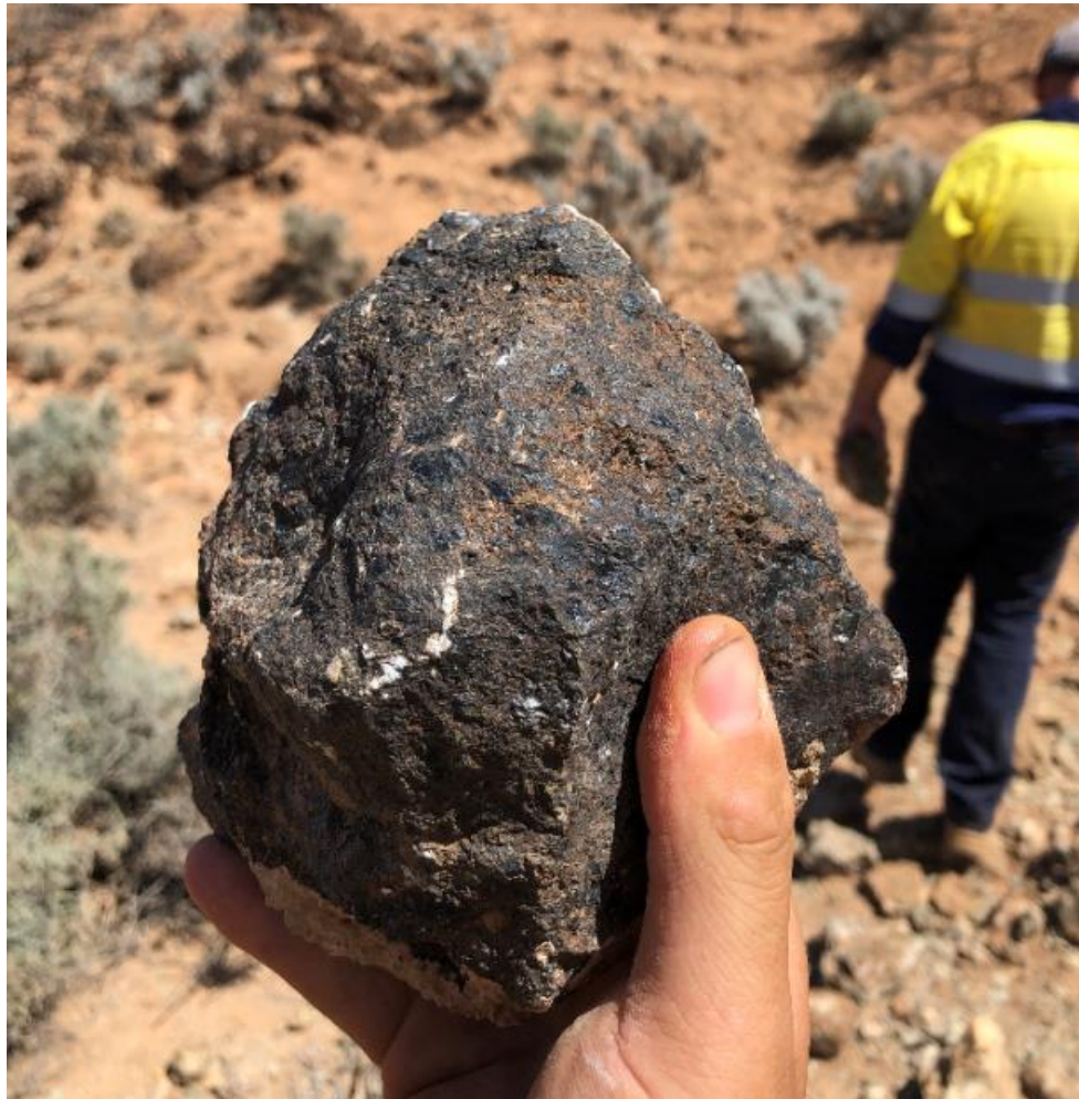
Figure 8: Sample TR004 – outcropping magnetite sampled at Torrens Project which returned anomalous Cu (0.9% Cu), Au (43ppb Au), Co (356 ppm Co) and V (1040ppm V).
